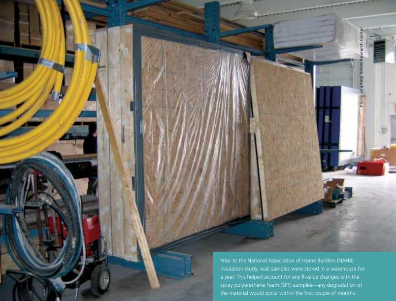
effect of the building shell under normal, realworld operating conditions are not considered in the R-value. This study is unique in its evaluation of overall wall system performance. It was designed to accurately characterize the energy consequences of wall construction and insulation material choices.
