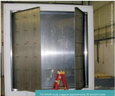
The NAHB study suggests approximately 85 percent more batt material than plastic insulation would be needed for a 88.9-mm (3.5-in.) cavity to achieve similar results.
